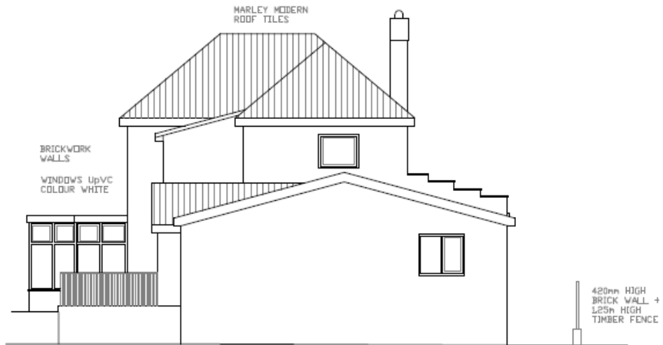
EXISTING SIDE ELEVATION
