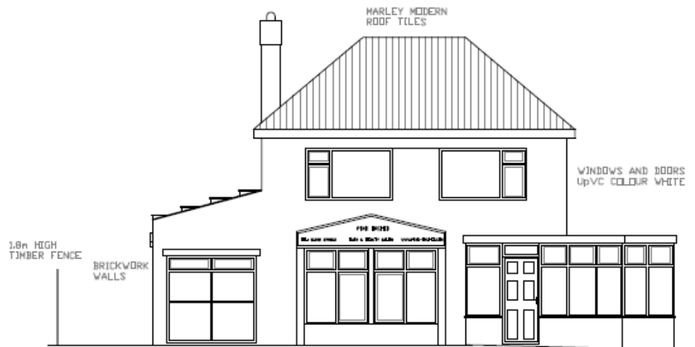
EXISTING SIDE ELEVATION
